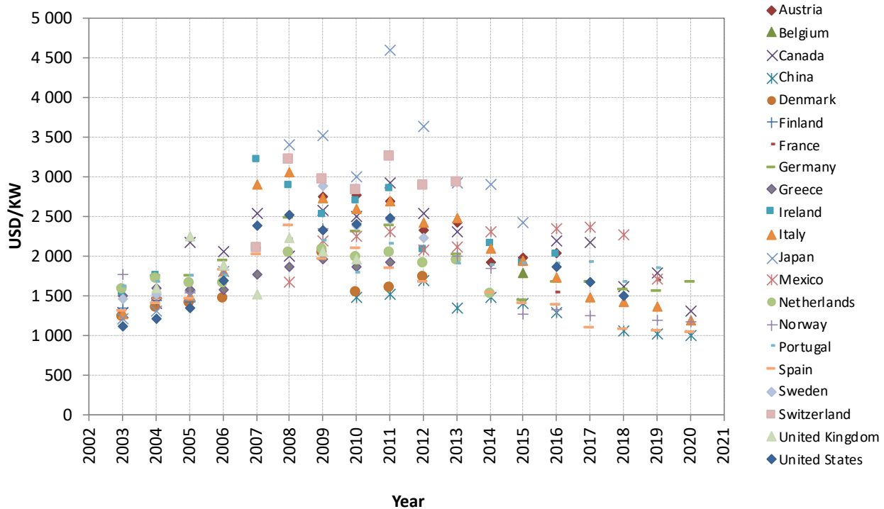
FIGURE 9. LAND-BASED WIND POWER PROJECT COST HISTORY FROM REPORTING IEA WIND TCP COUNTRIES.
