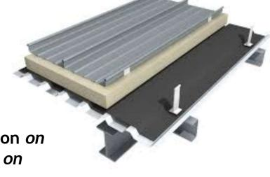
Metal Deck *on* Open cell insulation *on* Single membrane *on* Support Deck
