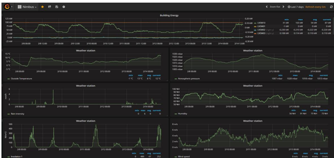
Figure 6: Example of BlockMeter Energy Dashboard for the Nimbus building Main Electricity Meter
