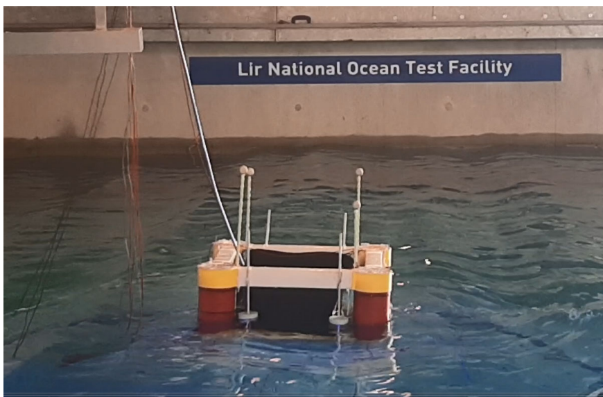
Fig Error! No text of specified style in document..5 OARPS Experimental modification: wave energy converter absorbers stability and dynamic tests.
