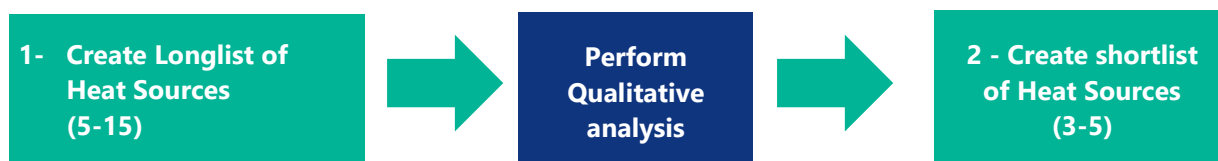
Figure 16: Outline Process to identify 1) an initial long list of options, perform a qualitative analysis on the longlist and b) identify as a result, a shortlist of heat sources.
