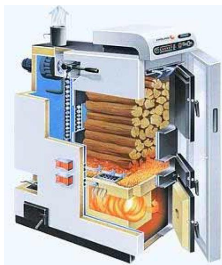
Figure 5.7: Overfed, under fire boiler 116
