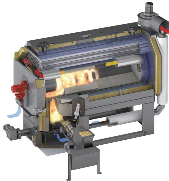
Figure 5.10: Overfed moving grate rotary combustion chamber boiler 69
