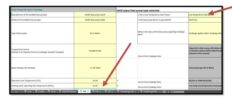
Entries related to heat emitters, backup heating, heat pump operation limit temperatures etc. all use the same approach as heat pumps assessed directly within the DEAP software following DEAP Appendix G. Note that for a Low Temperature heat pump, the unit is designed for lower emission temperatures (e.g. underfloor heating or system with radiators designed to run at a lower temperature). The entries for the example in question are as follows:
