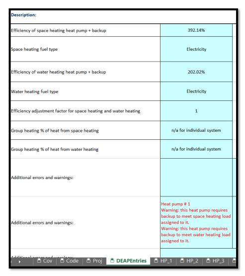
The space heating heat pump is entered in DEAP as an electric boiler as shown in Section 3.3.1. The water heating heat pump is as follows in DEAP:
