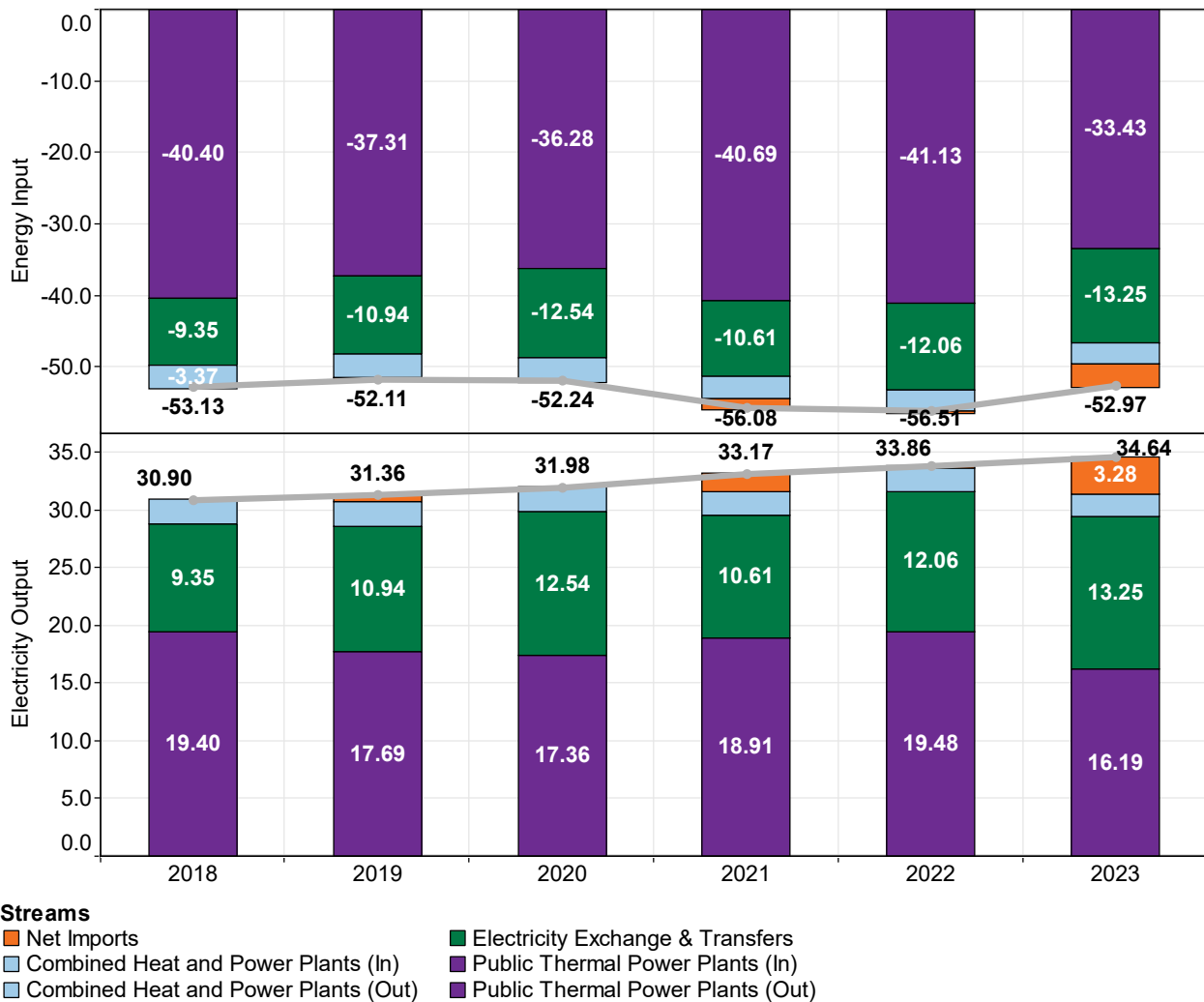
Energy Input to and Electricity Output from Electricity Generation (TWh) By Stream (Including Electricity Net Imports)
