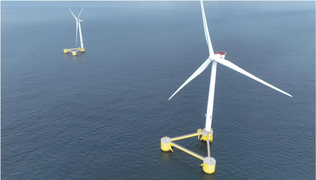
Figure 9: Example of a semi-submersible floating substructure. Photo of the WindFloat Atlantic project courtesy of Principle Power/Ocean Winds
