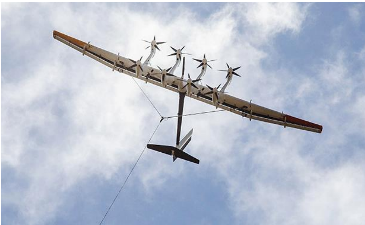
Figure 26: The Makani drone – an example of a rigid-wing, airborne-generating device. From Google's X, The Moonshot Factory
