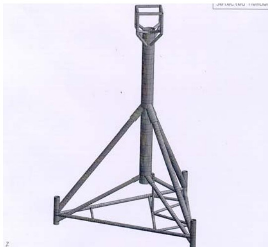
Figure 2. Tripod (piles not shown). The shown tripod is for the oil & gas sector, however, the design is equally relevant for an offshore wind turbine. Ref [11].
