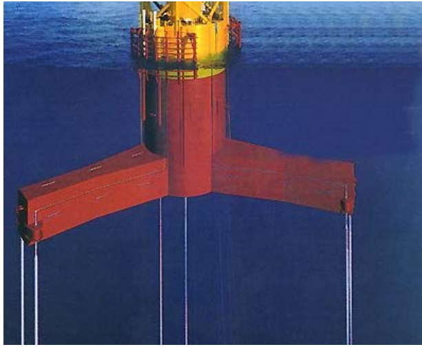
Figure 6. Floating support structure – tension leg type. Ref [11].
