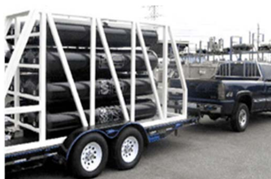
Figure 8. A BioCNG tube trailer. CNG at 250 bar occupies around 4 times the volume of the amount of diesel with equivalent energy content.
