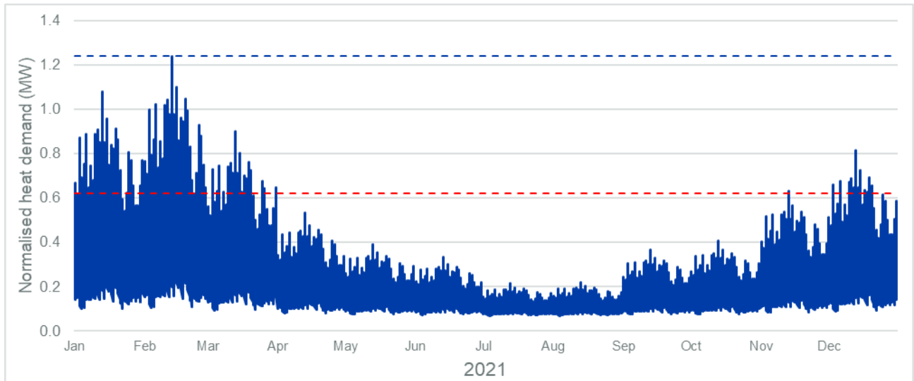
Figure 10: Annual normalised heat demand profile, based on imported profile shape from similar project. The dotted lines represent the peak demand (blue, 1.2MW) and 50% of the peak demand (red, 0.6MW)
