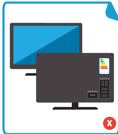
Incorrect location of energy label (i.e. rear of product)
