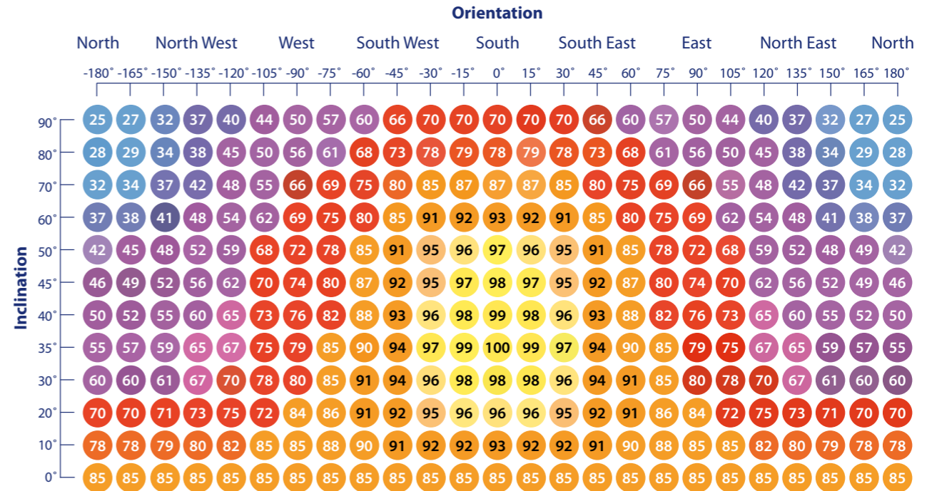
Figure 22: Solar PV output at varying orientations and tilts
