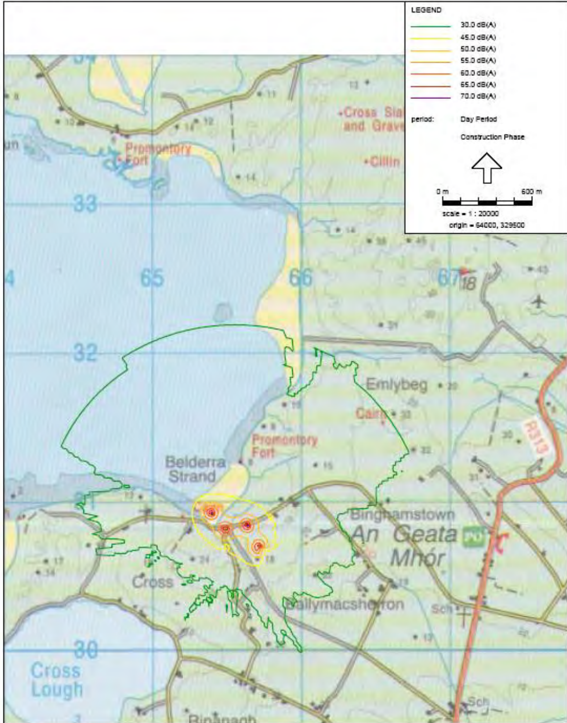
Figure 10-3: Construction phase predicted noise map
